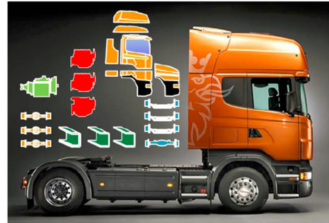
Figure 25: Effect of modularization on number of parts for a Scania truck cab [4] (Credit: Scania).
